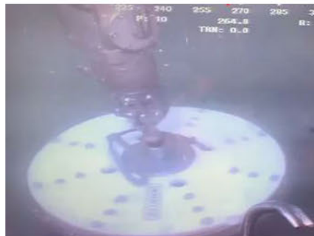
Polishing internal seal face
