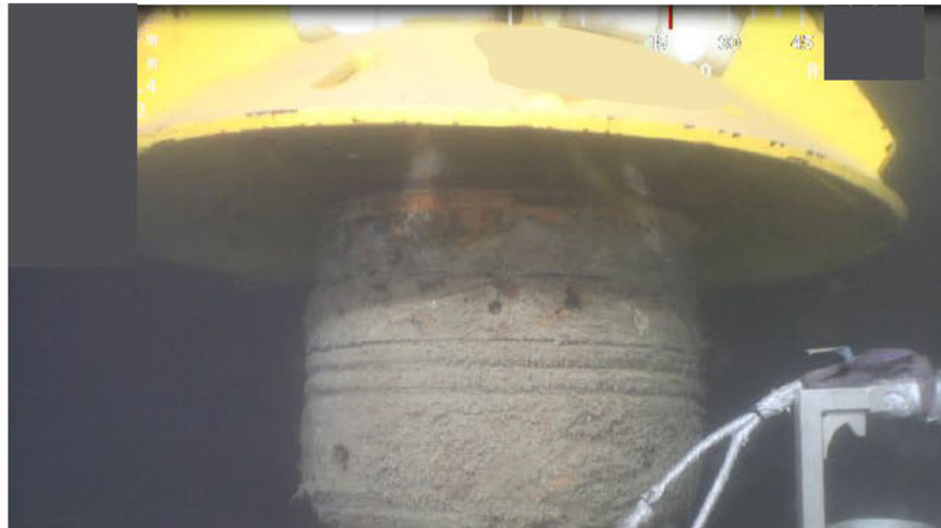
Latching Anchois-1 with Stena Don BOP
