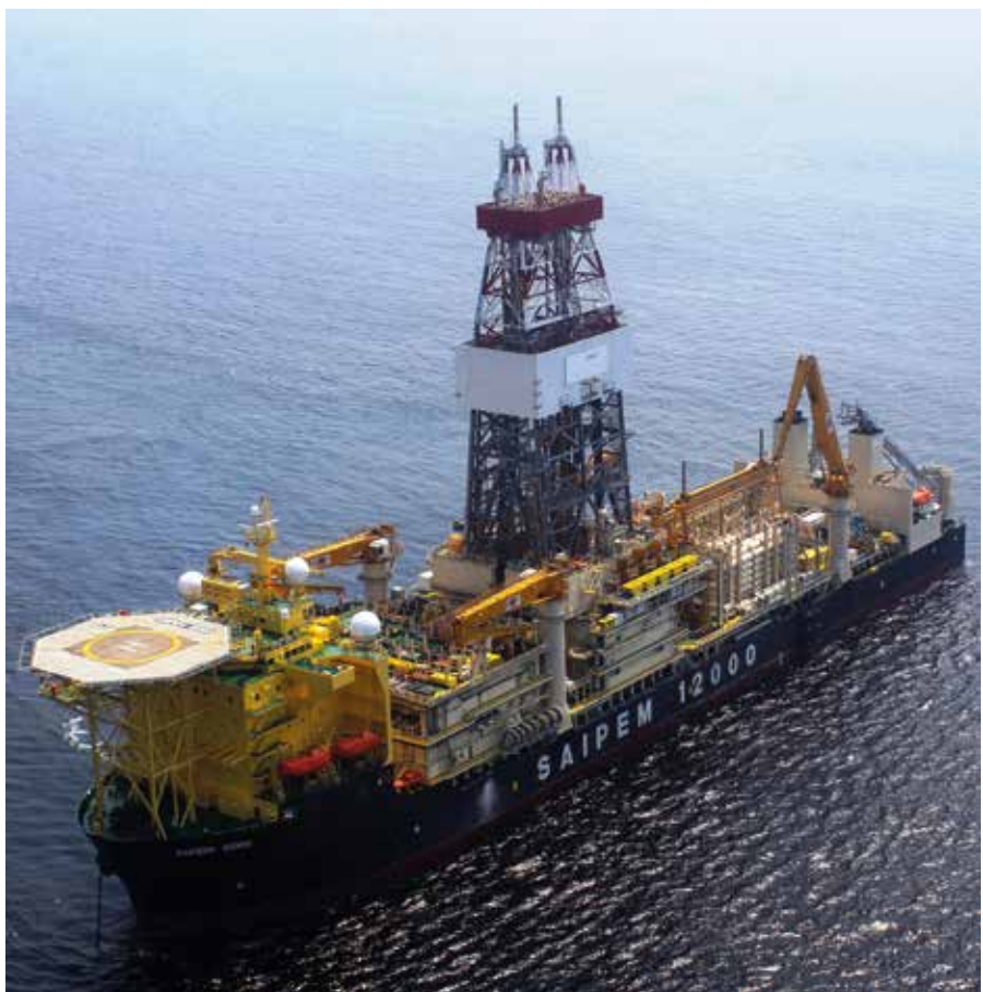
The Saipem 12000, a sixth generation ultra-deepwater drillship, was used to drill the Rabat Deep 1 well in Q1 2018.
