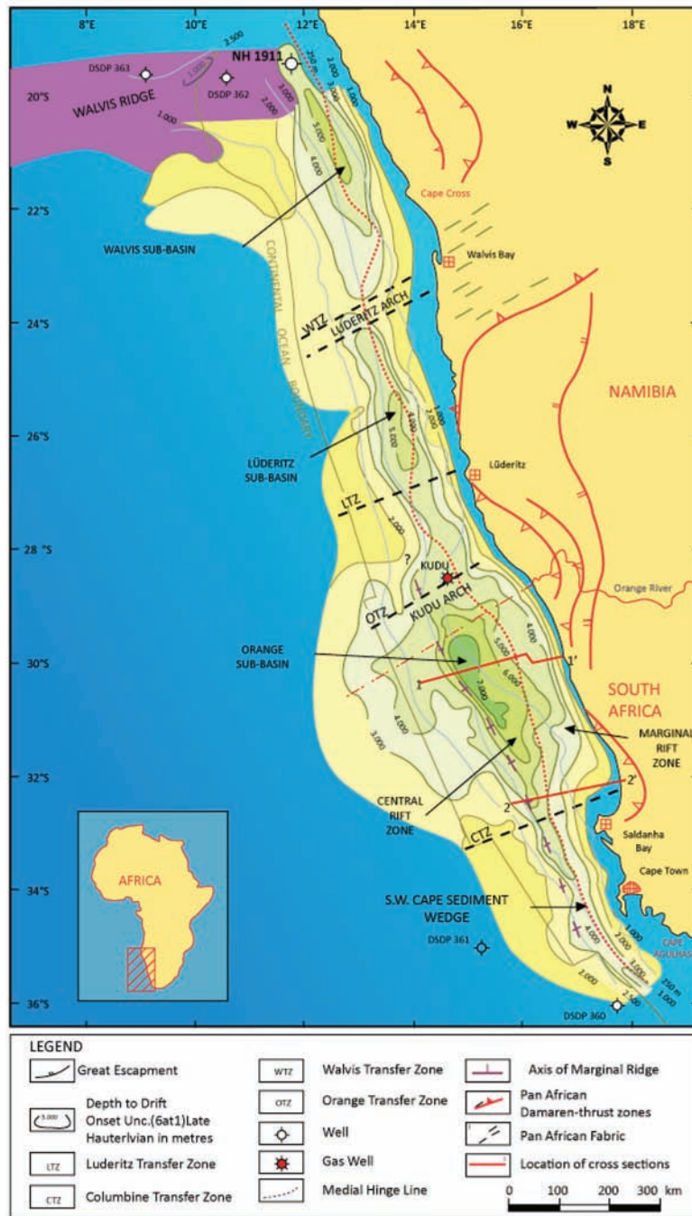
Figure 7 – Map of the Southwest African offshore basins with the main structural framework and sediments depocenters of the Walvis, Lüderitz and Orange Basins (Modified from Gerrard & Smith, 1980).
